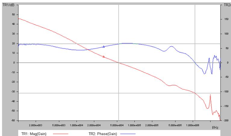
Figure 3: Bode plot of a stabilized switching regulator
